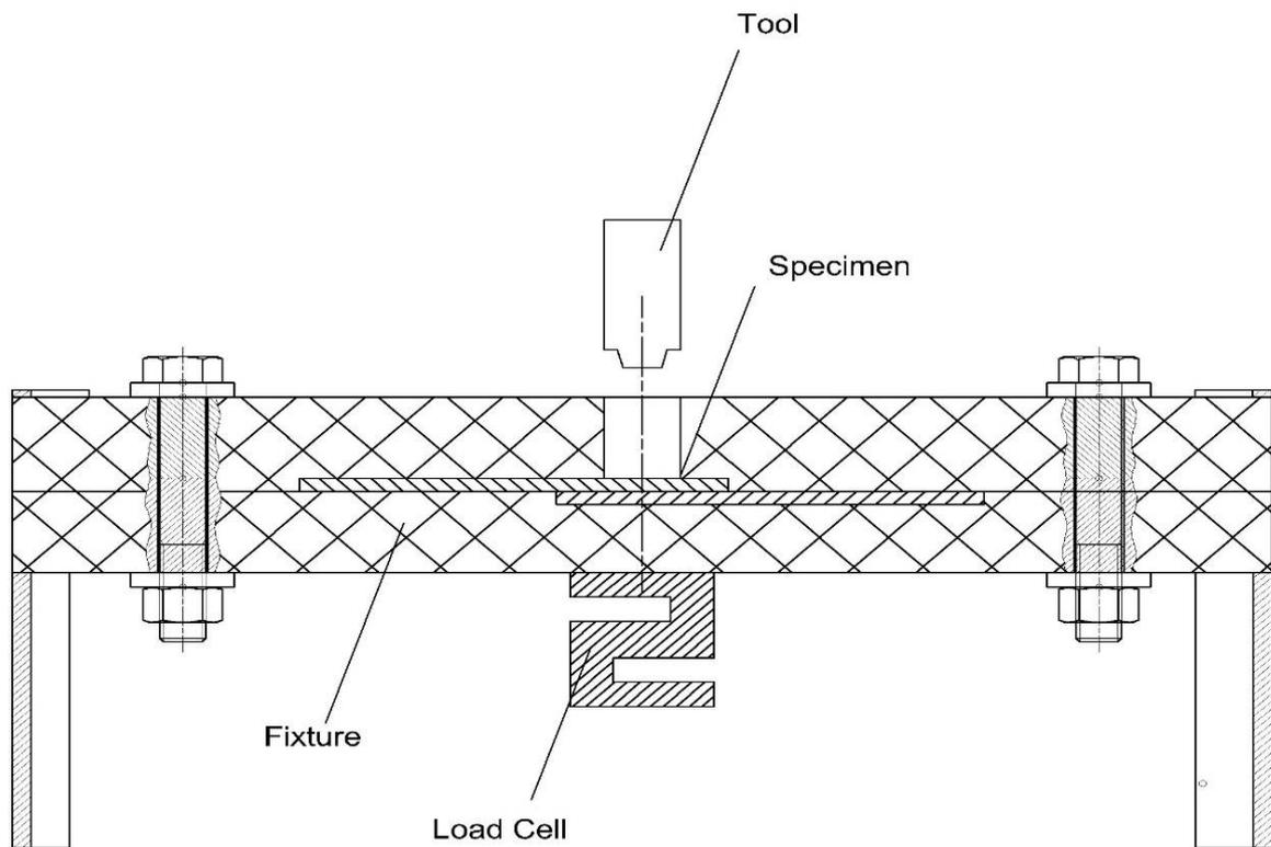
**Fig. 4 (b) Sectional view for force measurement set up**
