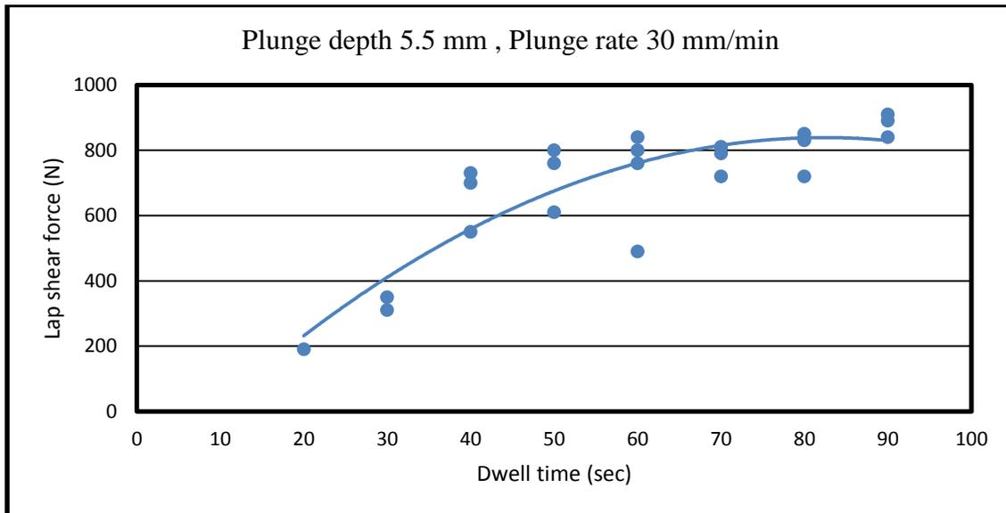
**Fig. 11 Effect of dwell time on lap shear force at tool rotating speed 1350 rpm**
