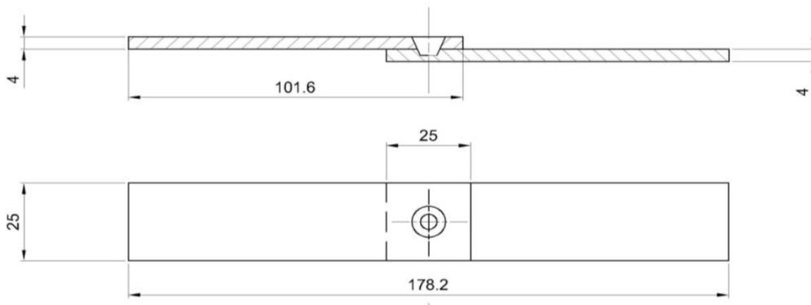
**Fig. 1 FSSW test specimen**
