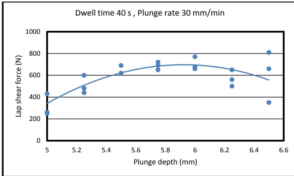
**Fig. 9 Effect of plunging depth on lap shear force at tool rotational speed 1350rpm**
