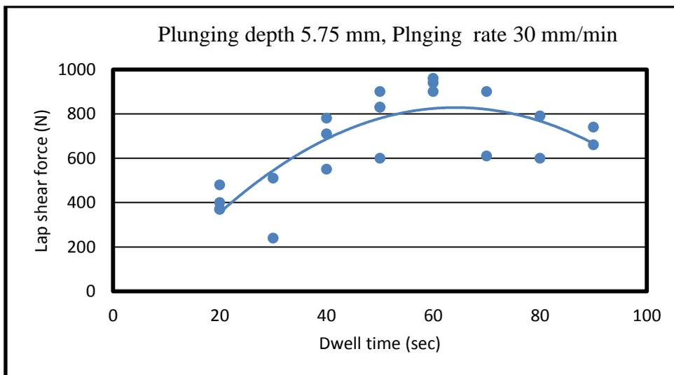
**Fig. 10. Effect of dwell time on lap shear force at tool rotating speed 2050 rpm**
