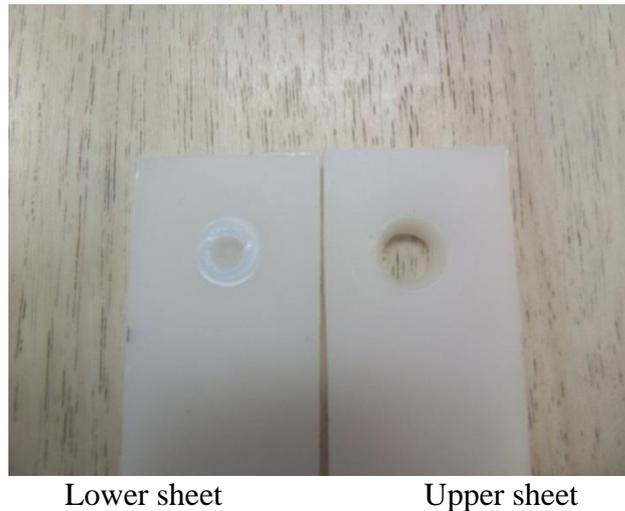
**Fig. 16 (b) Pull out nugget with lap shear force = 900N**
