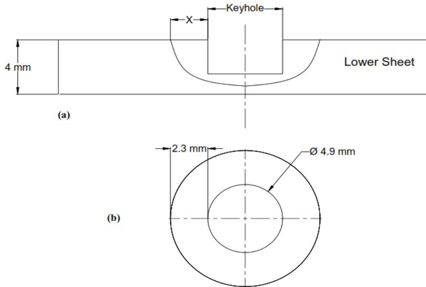
**Fig. 15 (a) Schematic illustration of the cross section of FSSW joint and (b) geometry of the weld bonded area, x: nugget thickness**
