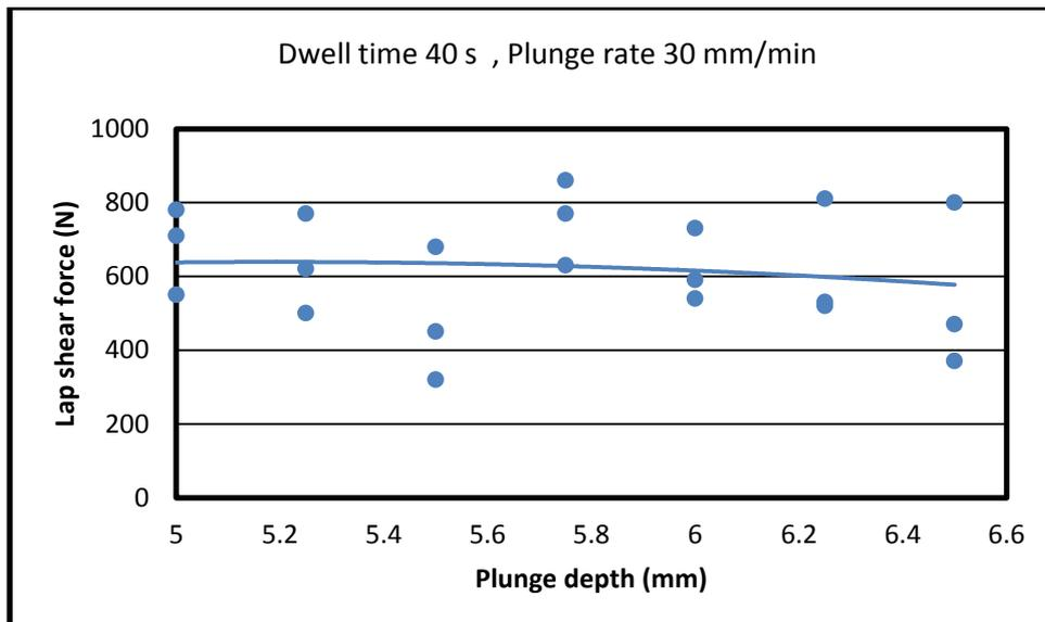
**Fig. 8 Effect of plunging depth on lap shear force at tool rotational speed 2050rpm**
