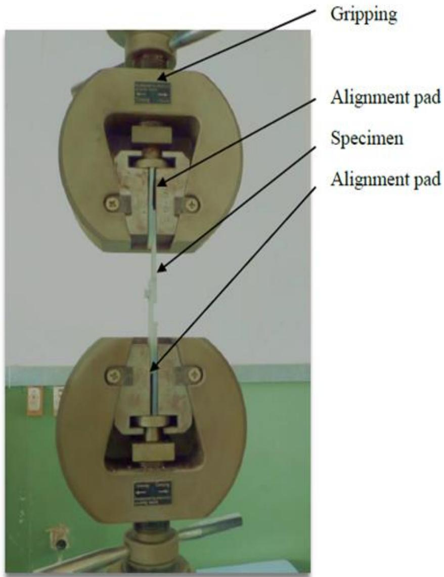
**Fig. 5 Lap shear test**
