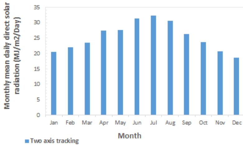
**Figure (3) Monthly mean daily direct solar radiation for two axis tracking system in Aswan**
