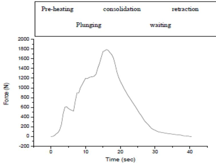
**Fig. 6 Plunging force during FSSW.**
