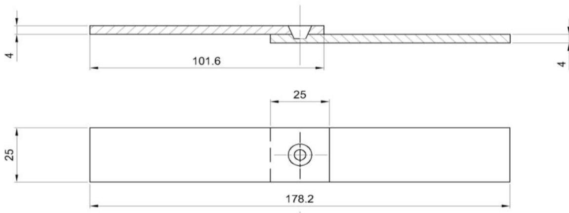
Fig. 1 FSSW test specimen
