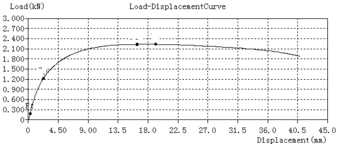
**Fig. 13 Load- displacement diagram of base material**
