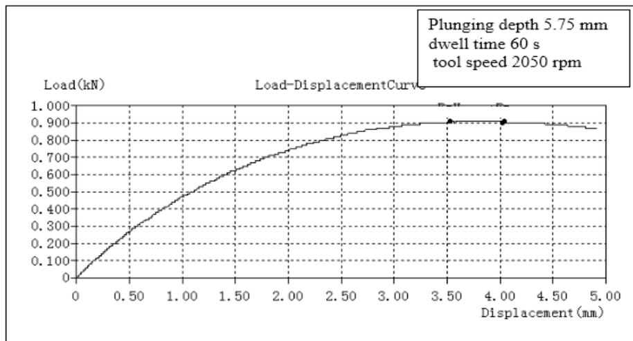
**Fig. 14 Load- displacement diagram of lap shear welded specimens**
