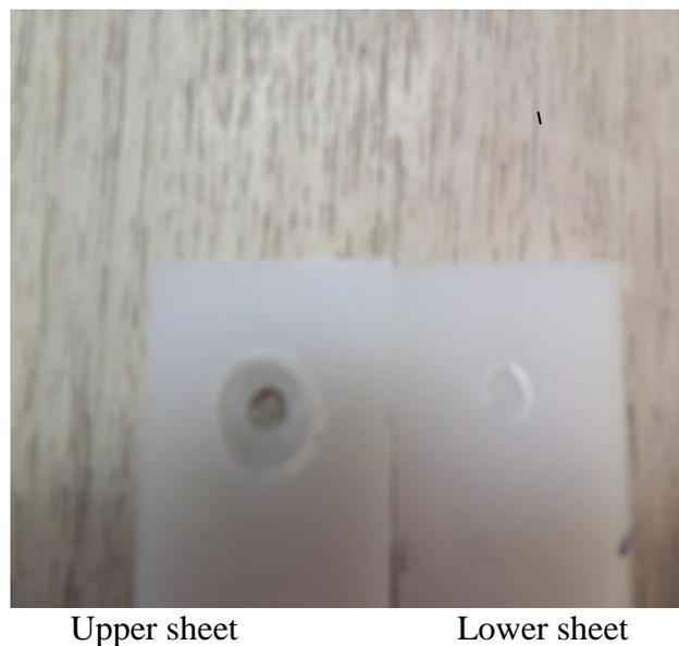
**Fig. 16 (a) Cross nugget with lap shear force = 240 N**
