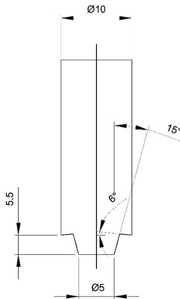
**Fig. 3 Tool geometry**
