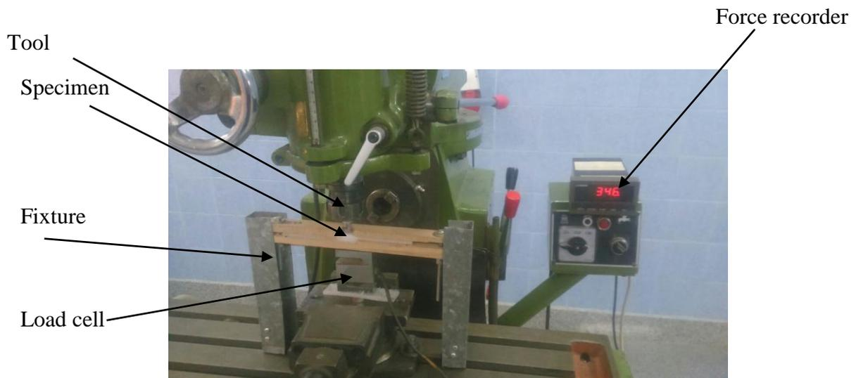
**Fig. 4 (a) Force measurement set up**
