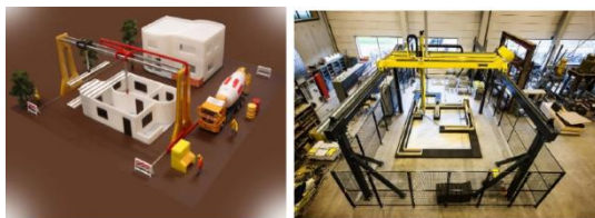
Fig. 5 Framed concrete 3D printers Source: https://www.tue.nl/en/university/departments/built-environment/research/research-programs/structural-design/research/research-areas/concrete-research-
